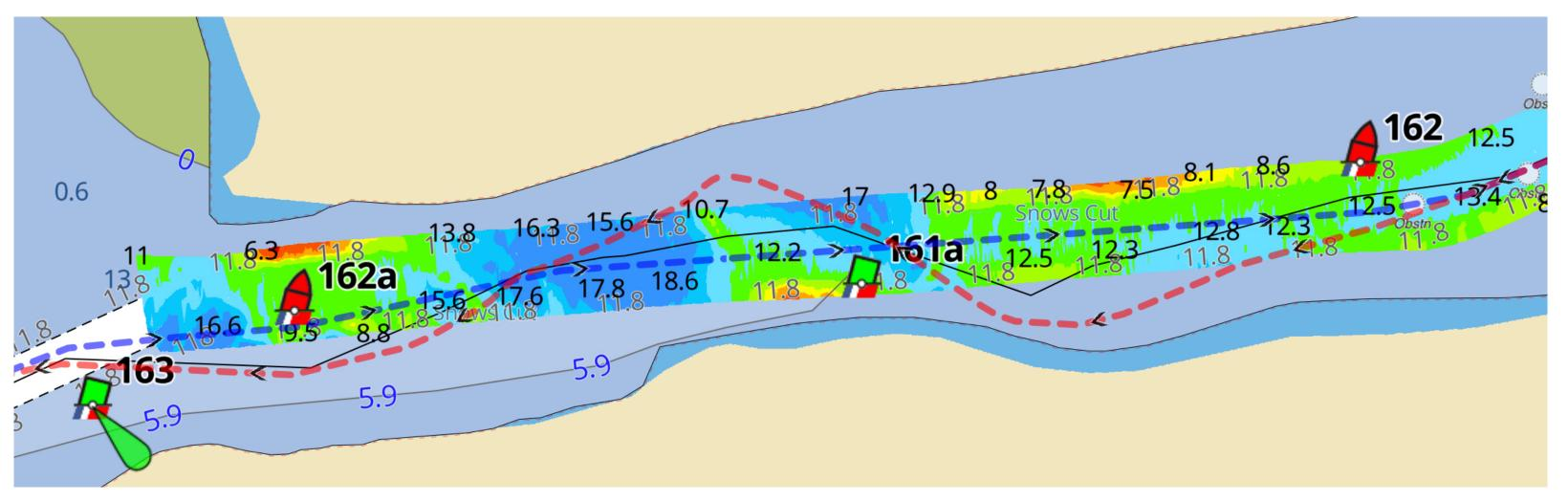
When a new **USACE** survey is completed, I adjust the Bob423 track to follow the newly dredged channel as verified by the survey.
